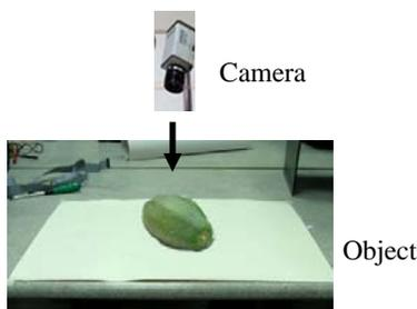
Fig. 2. Configuration of capturing images of papaya
