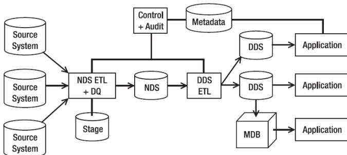
Fig. 1. NDS + DDS data flow architecture
